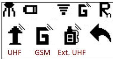
Figure 9: Receiver RTK Options
