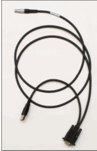
Figure 21: Serial Cable
