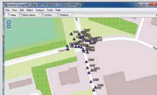
Stop and Go rover points for topo survey
