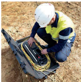
Carlson's Cabled Boretrak system is supplied in a Peli-case that can be hand carried by a single operative.
