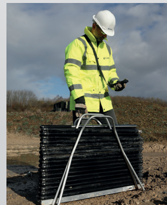
Rodded Boretrak's rods guide and locate the probe.
