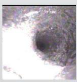
The nosecone camera provides a helpful view into the borehole during deployment.
