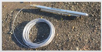
Boretrak2 probe with steel cable supplied for downhole deployments
