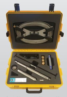
Boretrak2 system with 50-meter cable and RT4 Windows Tablet
