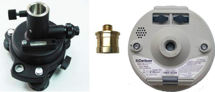
Figure 2-5: Installing BRx6 on a Tribrach
