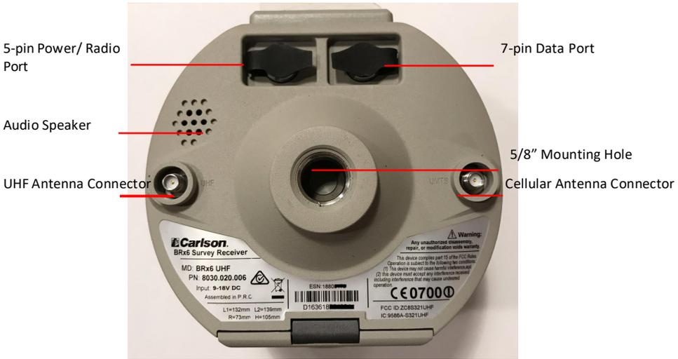
Figure 2-1: BRx6 ports and connectors
