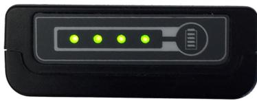
Figure 2-3: Fully Charged Battery Indicator
