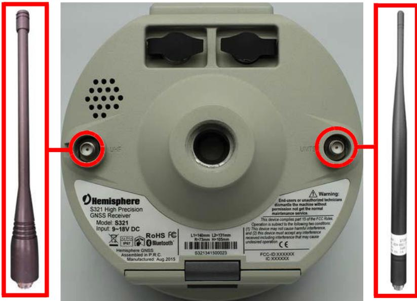
Figure 2-4: Installing UHF and GSM Antennas
