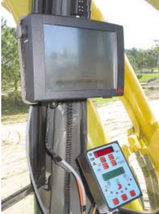
Simple Mikrodigger controls at lower right — the DigStar computer display is above, and can easily be removed along with GPS and radios in pelican case (above).
